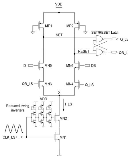
Fig .4. Low Swing Differential Conditional Capturing Flip Flop
