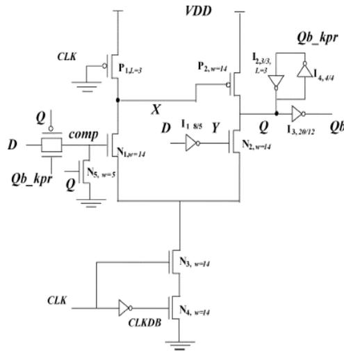
Fig .7.Clocked Pair Shared Flip Flop
