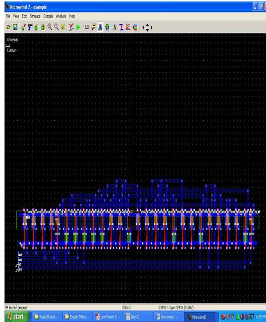
Fig.5.LSDCCFF Layout in microwind
