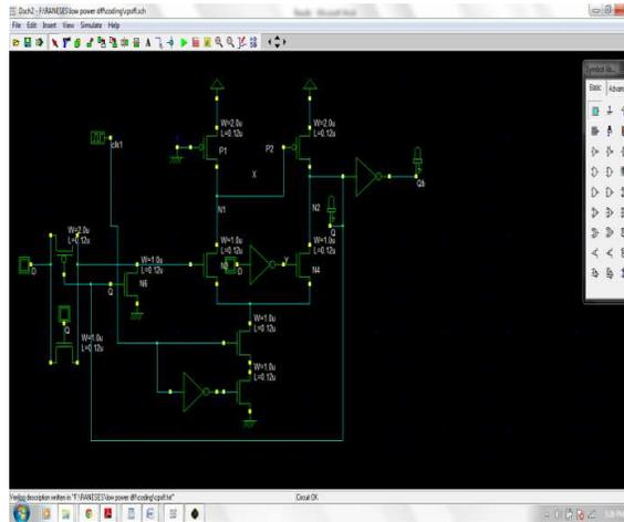
Fig.8. Execution of the Clocked Pair Shared Flip Flop
