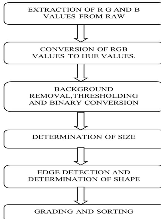
Fig 1 Steps Followed In Image Processing Using OpenCV
