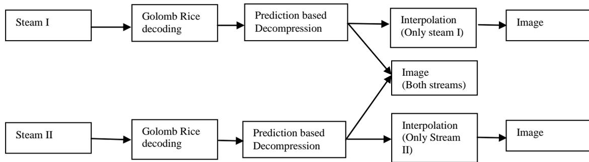
Fig. 5 Block Diagram of the Decompression Algorithm
