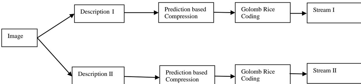
Fig. 4 Block Diagram of the Compression Algorithm
