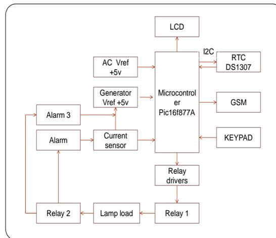
Fig1.functional block diagram of maximum demand control
