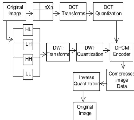
Figure.1.1.Architecture of DCT and DWT Comparison
