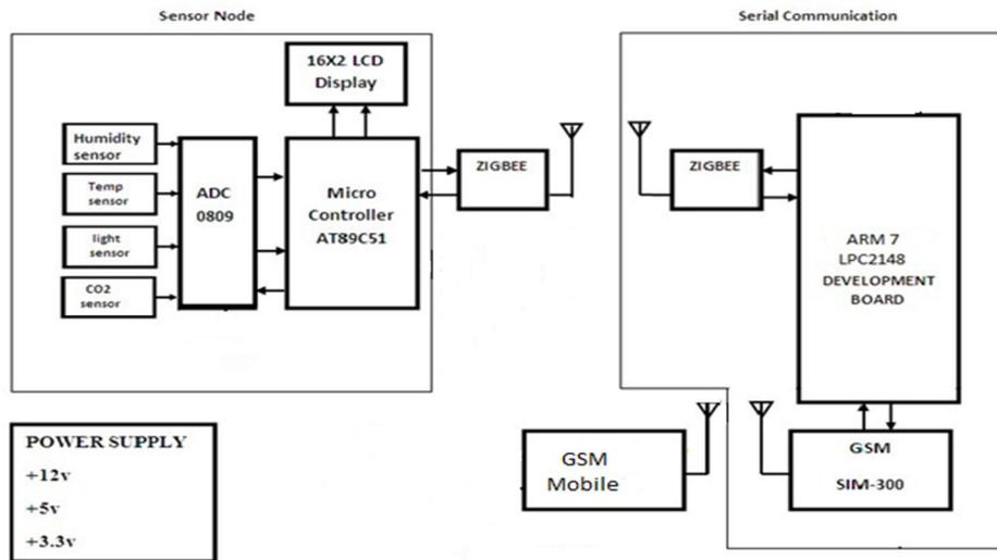
Figure1: System block diagram of the overall structure
