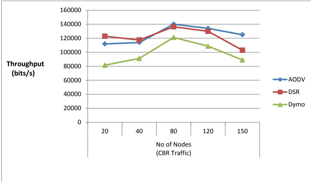
(Fig.2 Throughput Vs No. of Nodes for CBR Traffic)
