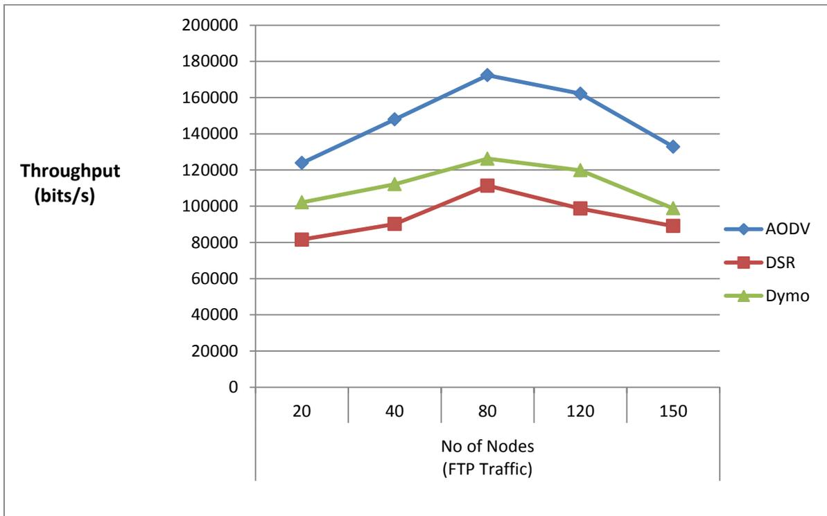
(Fig.3 Throughput Vs No. of Nodes for FTP Traffic)
