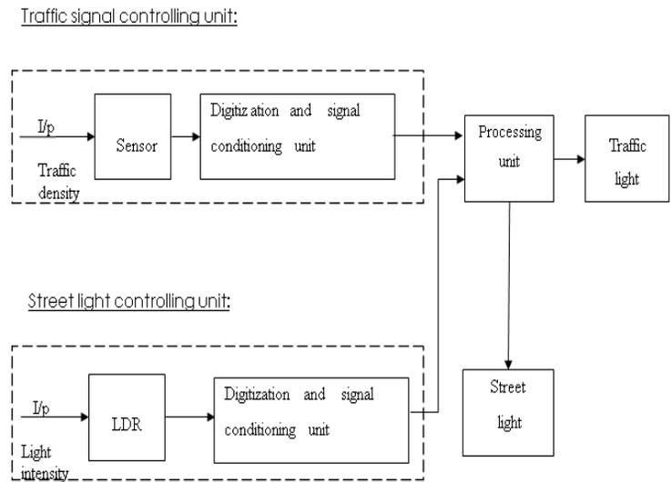
**Fig.1: Power Saver Street Lighting and Automatic Traffic Management System**
