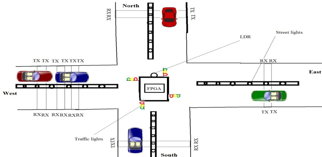
**Fig.2: Traffic Signal Controlling Unit**
