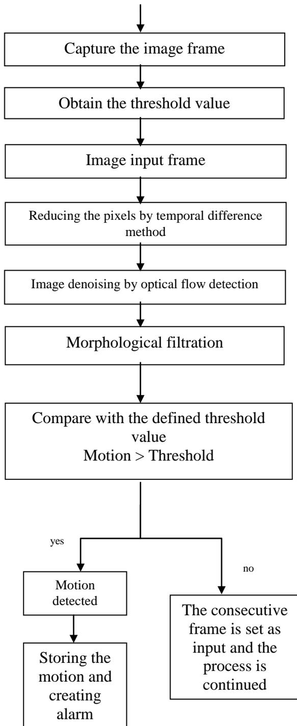
**Fig 1. Algorithm block diagram**
