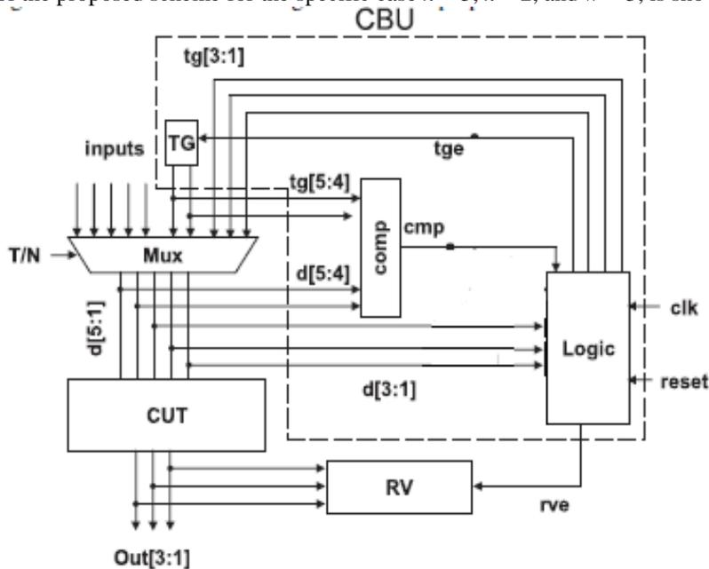
**Fig 3: Proposed architecture for  $n=5$ ,  $k=2$ ,  $w=3$ .**
