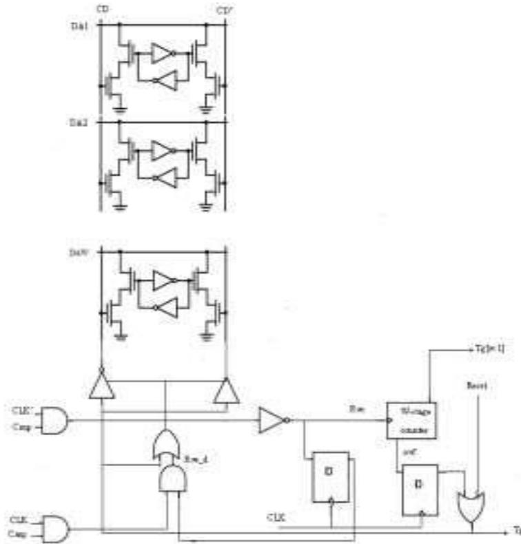
**Fig 4: Proposed logic module**
