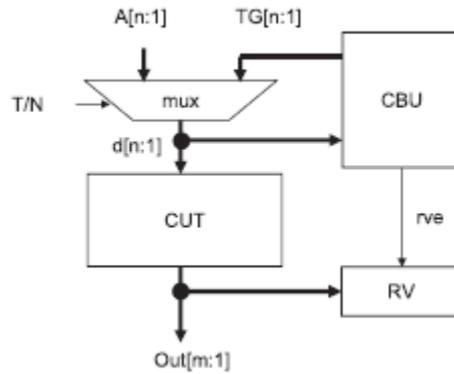
**Fig 1: Input vector monitoring concurrent BIST architecture.**
