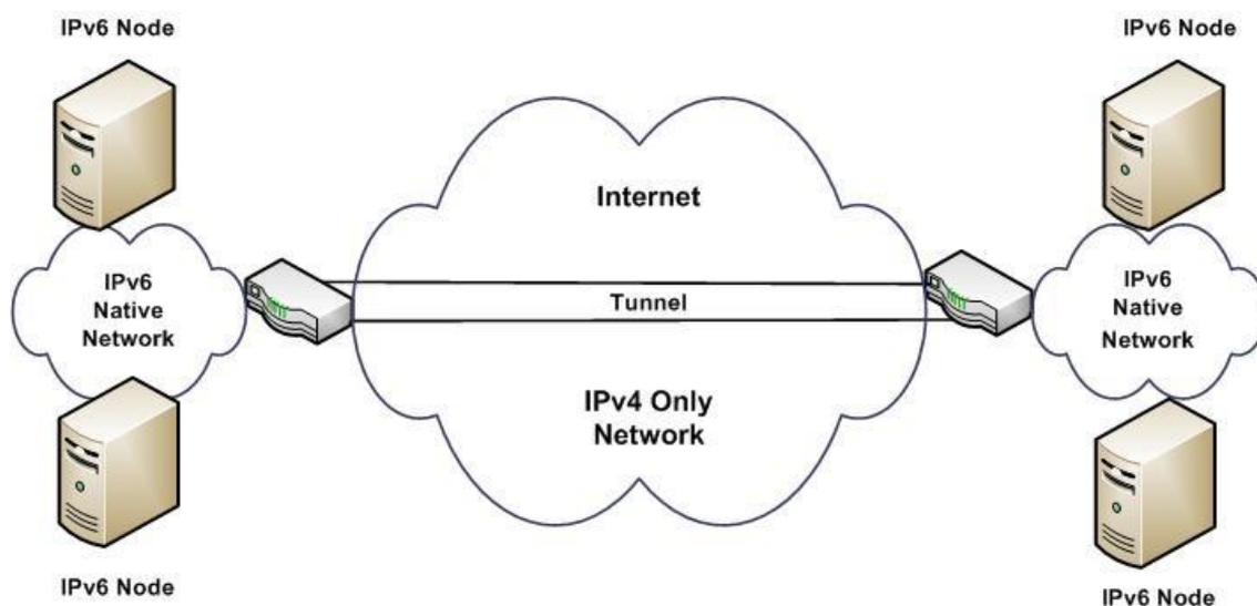
Figure 1 IPv6 Tunneling over IPV4 only network
