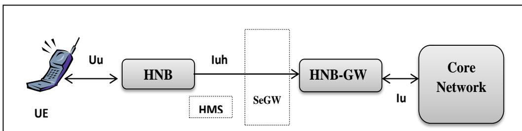
**Fig. 4** 3G Femtocell logical architecture
