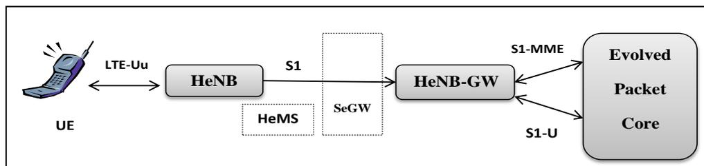
**Fig. 6** 4G Femtocell logical architecture
