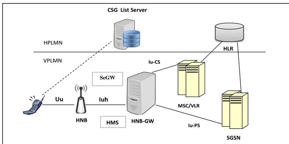
**Fig. 5** High-level functional architecture of 3G femtocell
