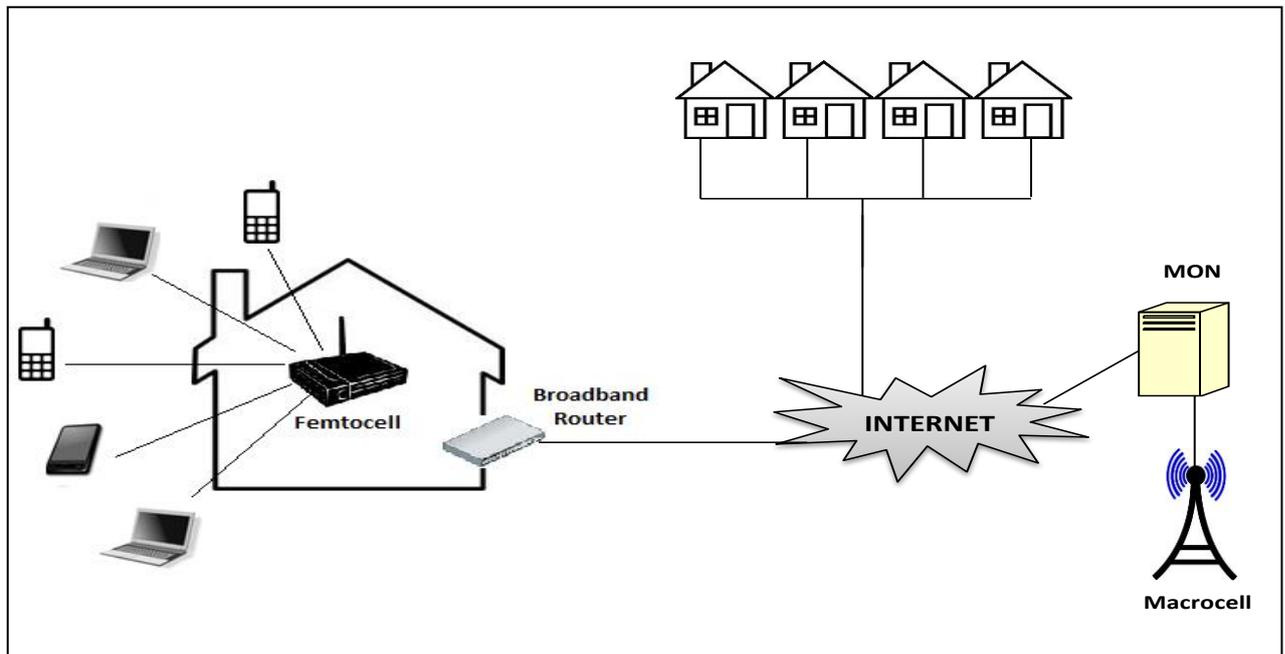
**Fig 3** Basic architecture of Femtocell
