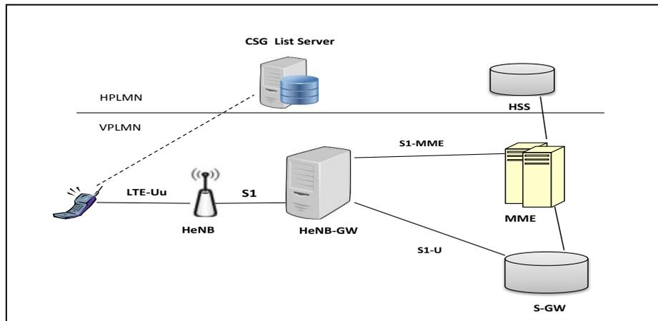
**Fig. 7** High-level functional architecture of 4G femtocell
