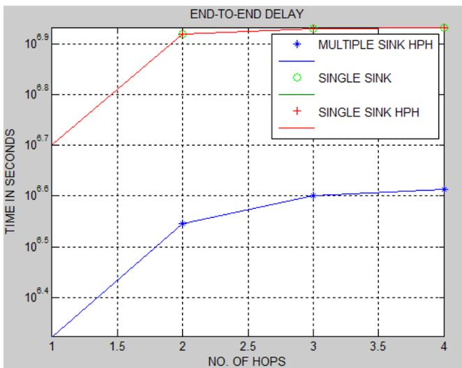
Figure 6: Average End-To-End Delays
