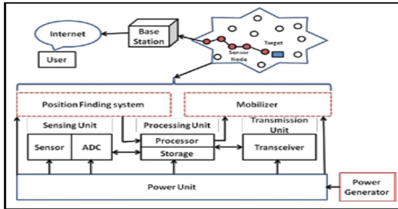
Fig. 2: Components of Sensor Node
