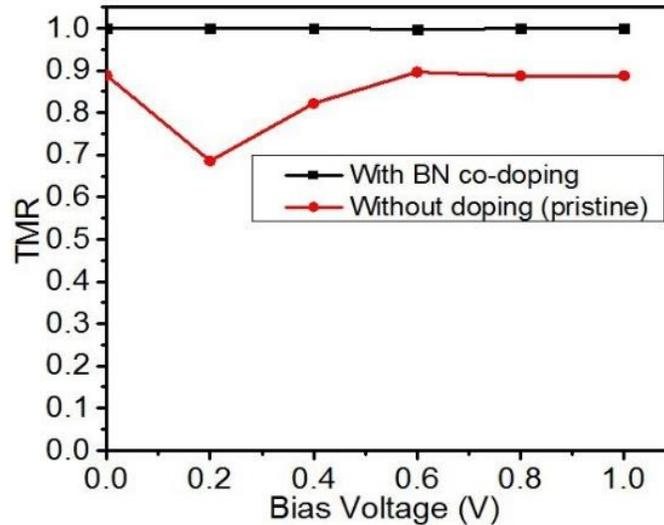
Fig. 4. TMR curves showing comparison between pristine and BN co-doped graphene based MTJ. High values of TMR  $\sim 100\%$  at all bias voltages in BN co-doped structure indicates perfect tunneling magneto resistance effect.
