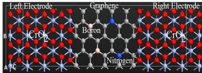
Fig. 1. MTJ consisting of BN co-doped graphene nanosheet sandwiched between CrO<sub>2</sub> (Left-Right) HMF electrodes.
