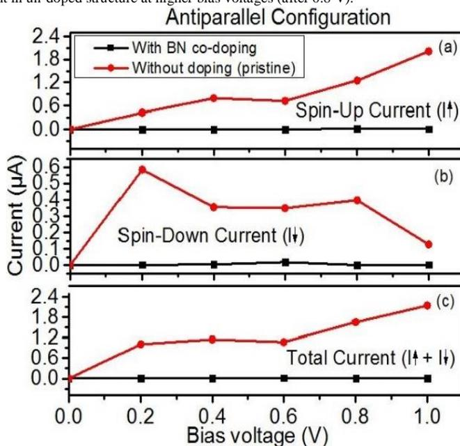
Fig. 3. I-V curves showing comparison of tunneling current between pristine and BN co-doped graphene based MTJ for antiparallel configuration (APC). (a)  $I_{\uparrow}$  is larger in un-doped structure. (b)  $I_{\downarrow}$  is larger in un-doped structure. (c) Total current (sum) is larger in un-doped structure.
