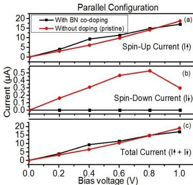
Fig. 2. I-V curves showing comparison of tunneling current between pristine and BN co-doped graphene based MTJ for parallel configuration (PC). (a)  $I_{\uparrow}$  in doped structure is slightly more than  $I_{\uparrow}$  in pristine (un-doped) structure in the bias range of 0 V to 0.8 V. (b)  $I_{\downarrow}$  is much larger in un-doped structure. (c) Total current (sum) in doped structure is slightly less than the current in un-doped structure at higher bias voltages (after 0.8 V).
