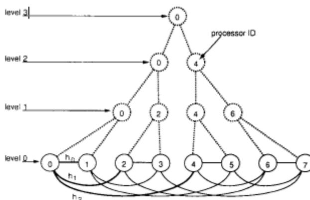
Fig. 2 Hierarchical organization of an eight-processor system with hypercube interconnections, where  $h_k$  is the connection to the neighbor at the  $k$ th level. The processor IDs at intermediate nodes in the tree represent those processors delegated to manage the balancing of corresponding lower-level domains.
