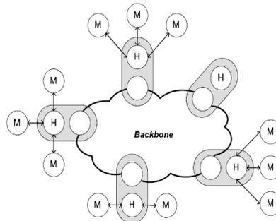
Fig: The structure of a protocol node in the B-CT protocol
