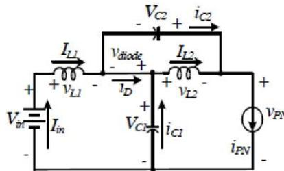
Fig.3.Equivalent circuit of QZSI in Active mode
