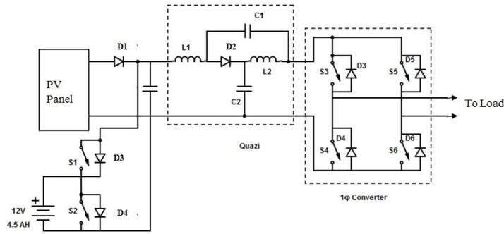
Fig.2 Optimized energy-stored qZSI for PV off-grid applications.
