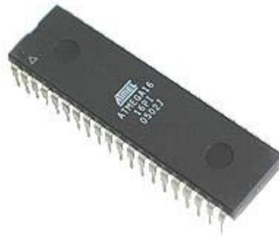
Figure 1 Microcontroller AtMega 16
