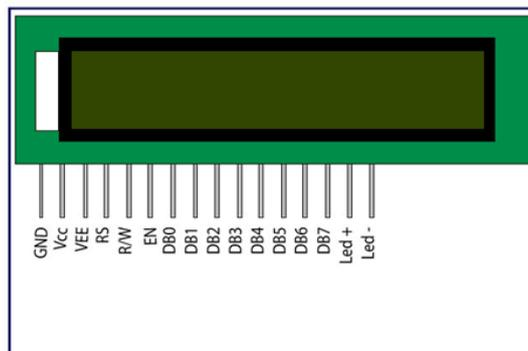
Figure 4 16x2 LCD display
