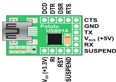
Figure 6 Serial to USB converter device
