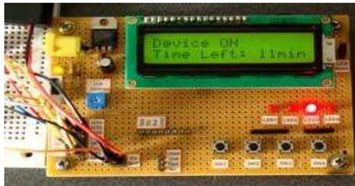
Figure No 4: Transformer Tripper
