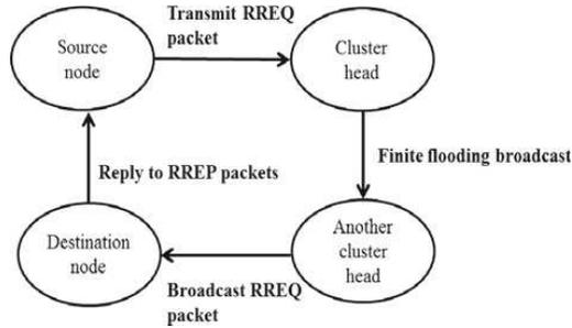
Figure 1: The state-transition diagram of Route discovery
