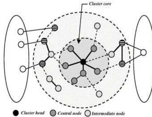
Figure 2: A cluster based ad hoc network
