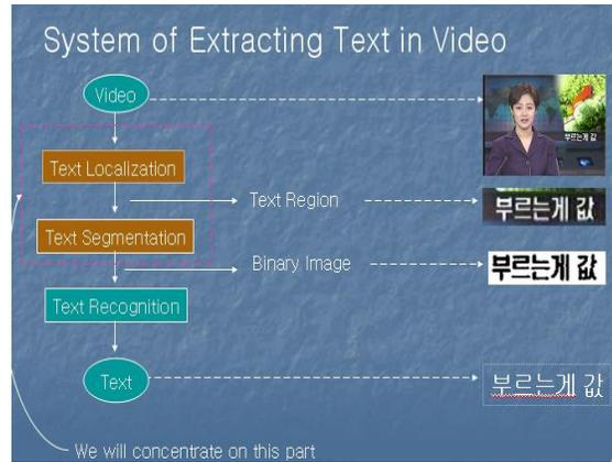
Fig IX Block Diagram For Text Extraction
