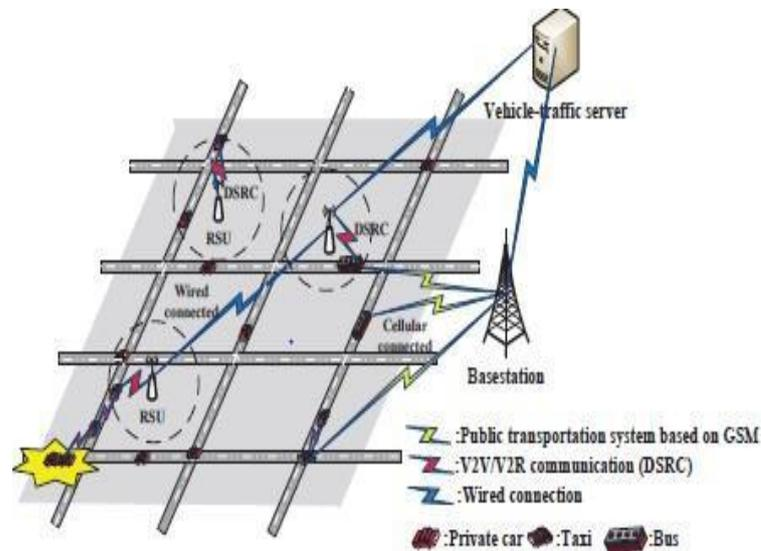
Fig .3 Hybrid VANET-enhanced network architecture
