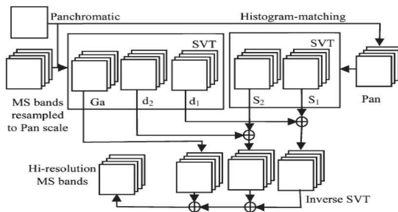
Fig. 2. Flowchart of an SVT-based fusion of MS and Pan data with 4 : 1 ratio.
