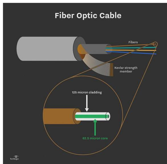
Multimode fiber is used for shorter distances because the larger core opening allows light signals to bounce and reflect more along the way. The larger diameter permits multiple light pulses to be sent through the cable at one time, which results in more data transmission. This also means that there is more possibility for signal loss, reduction or interference, however. Multimode fiber optics typically uses an LED to create the light pulse.
