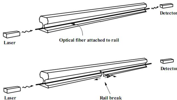
**Fig: Concept of rail break detection. During a rail break, the fiber bonded to the rail also breaks and light transmission through the fiber decreases dramatically.**
