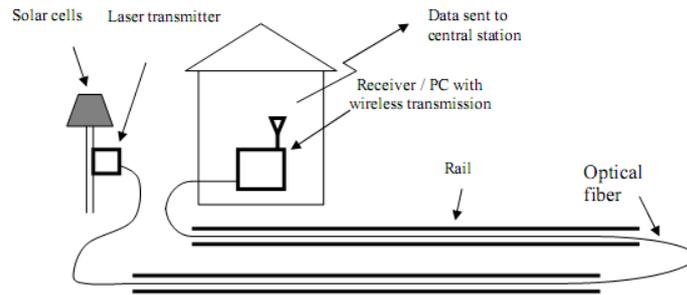
**Fig: Schematic of a complete fiber-optic sensor system which includes the laser transmitter, fiber-optic sensor, photo detector receiver, and data acquisition components including a modem for wireless transmission, computer, and data storage and analysis software.**
