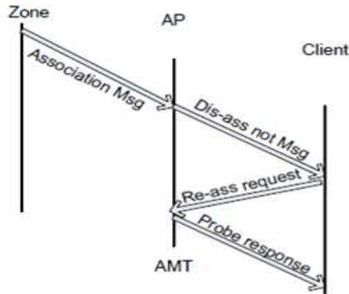
Figure 7. Message exchanged during the AMT phase
