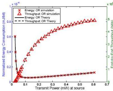
Fig. 4. The NEC  $\bar{E}_{total}$  and the end-to-end throughput  $R_{e2e}$  versus the transmit power  $P_{t_s}$ .
