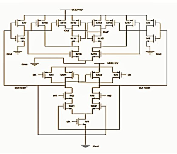
Fig 2. Proposed dynamic latch based comparator
