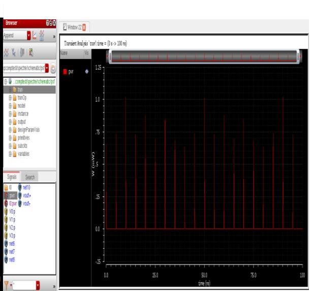
fig 4 Power dissipation of latch based comparator
