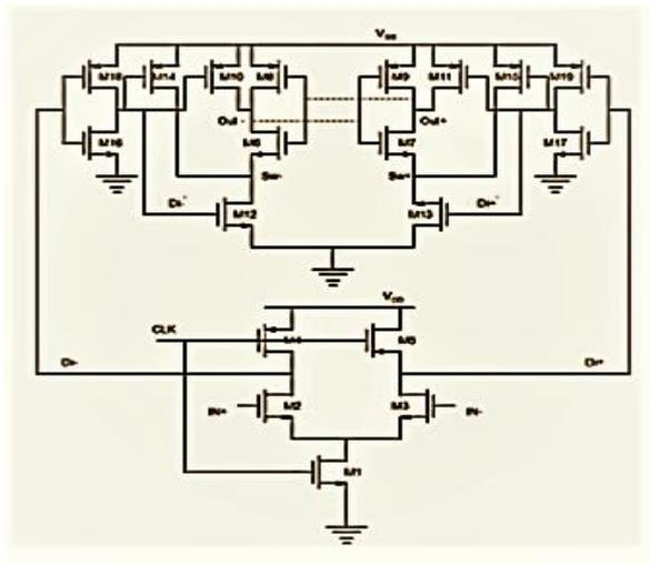
Fig No 1. Conventional latch based comparator
