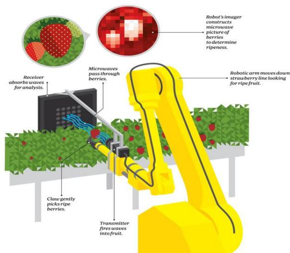
Figure-1 second prototype –strawberry fruit picking robot
