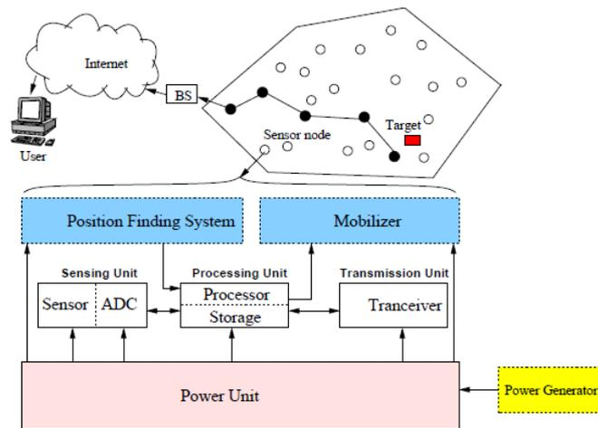
Fig 1: General components of Sensor nodes
