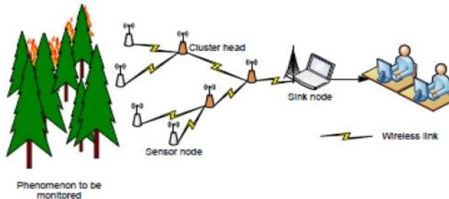
Fig 1. Architecture of Wireless Sensor Network
