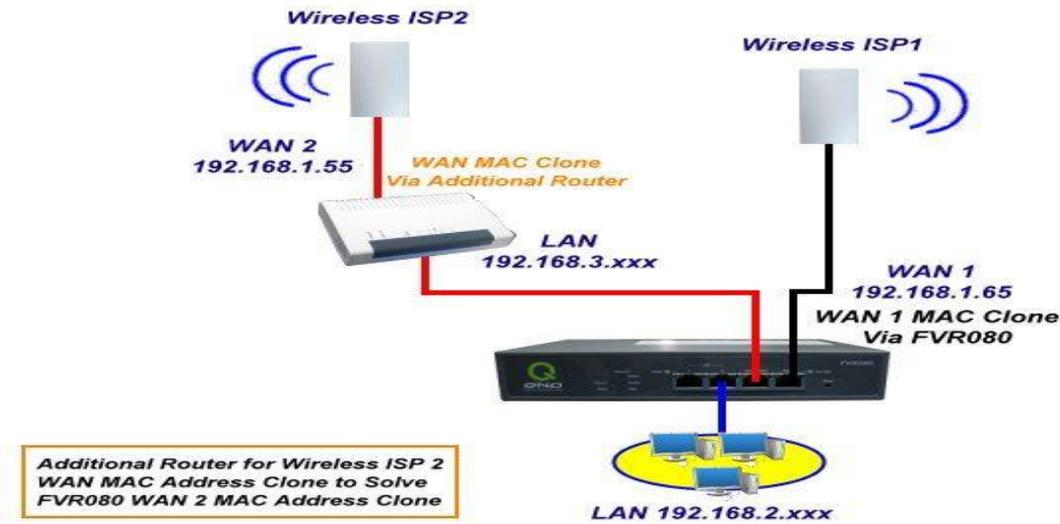
Fig. Illustration of MAC Cloning in Wireless LANs
