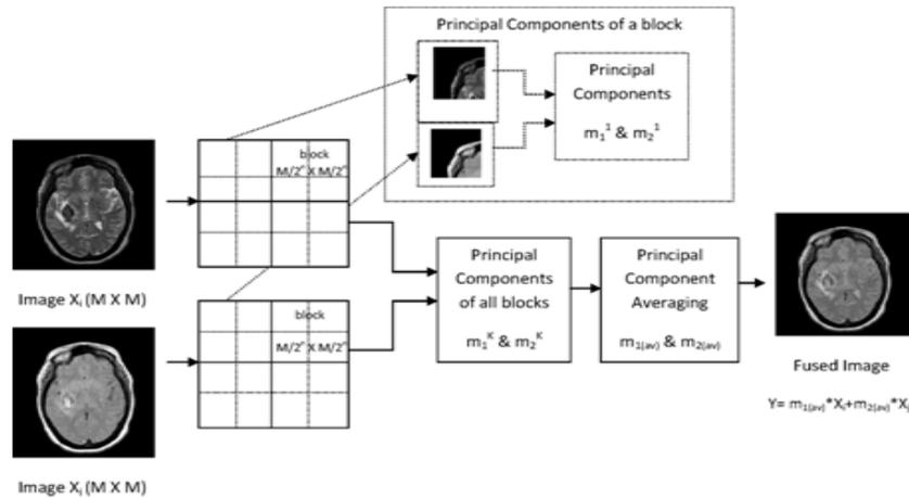
Figure 1: Block Diagram of Iterative Block Level Principal
