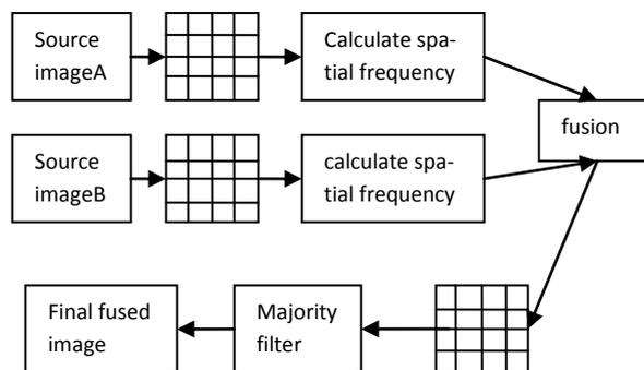
Figure 2: Block Diagram of image fusion process
