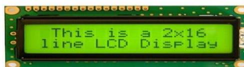
Fig 5 LCD display
