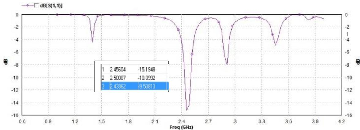
Fig. 3(a). Reflection coefficient (s11) of hexagonal patch.
