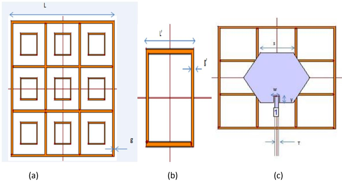
Fig.2.(a) EBG structure on felt substrate, overall size of EBG is 116x116 mm and inner gap (g)=2 mm. (b)each cell dimension is  $L'=19 \times 19$ mm and  $g'=2$ mm (c)  $S=32.6$ ,  $W=6$ ,  $X=20$ ,  $Y= 6.5$  and  $T= 3.9$
