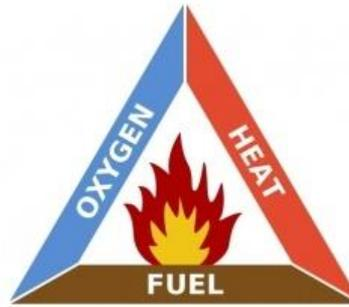
Fig. 1 Fire triangle diagram.
