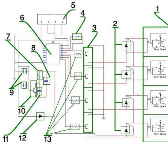
Fig. 3 The diagram of radio receiver circuit.
