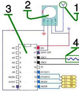
Fig. 4 The diagram of radio transmitter circuit.
