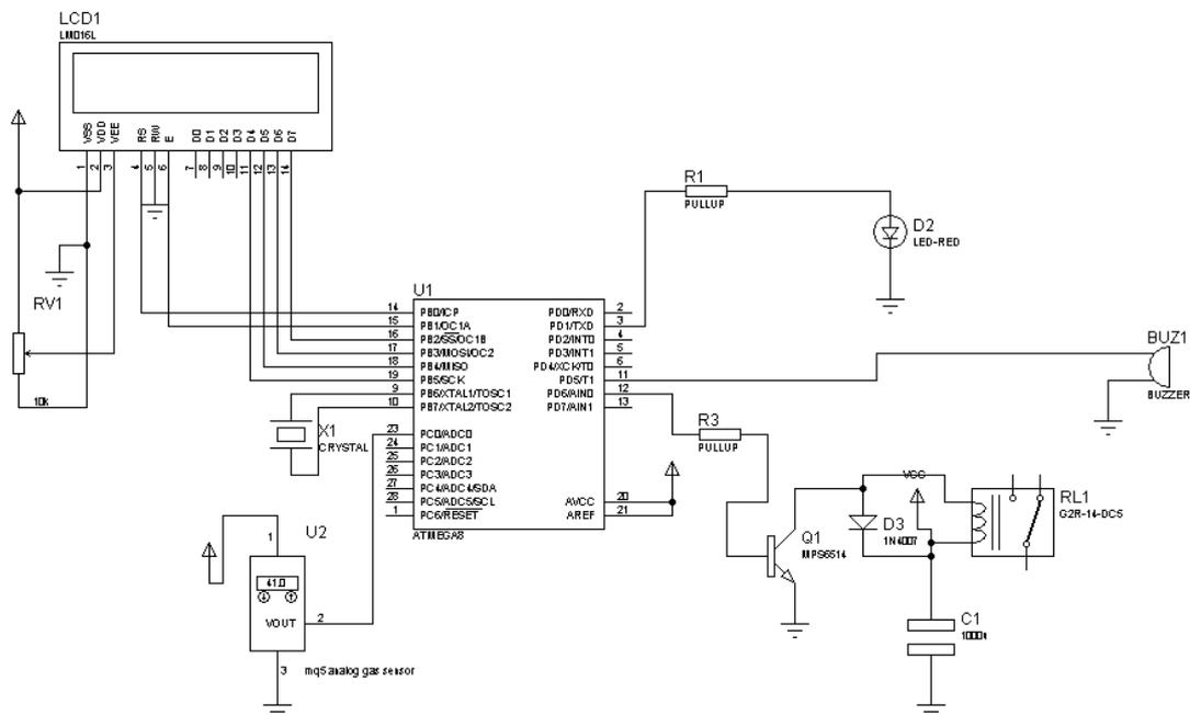
Fig. 2 Circuit diagram of an intelligent system for detecting of gas emissions.
