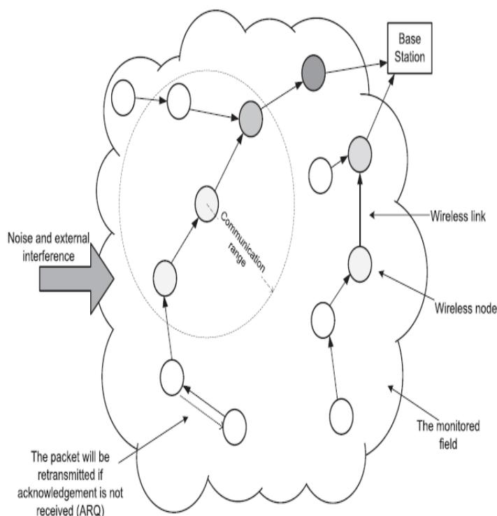
Figure 1 Wireless sensor network.
