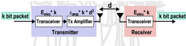
In order to transmit k-bit message over distance d, energy used is-
