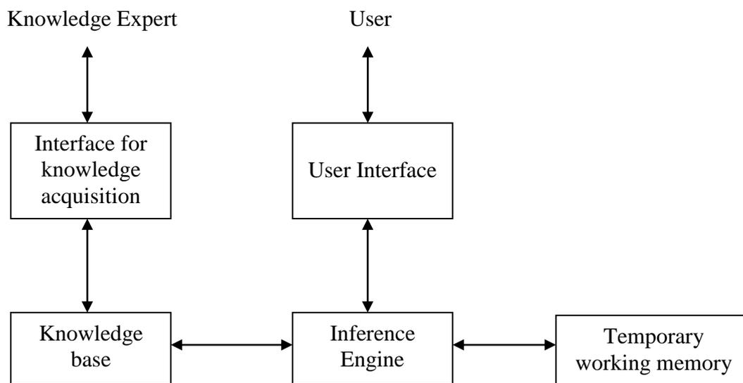
Figure 1: Components of Rule-Based Expert System<sup>[8]</sup>
