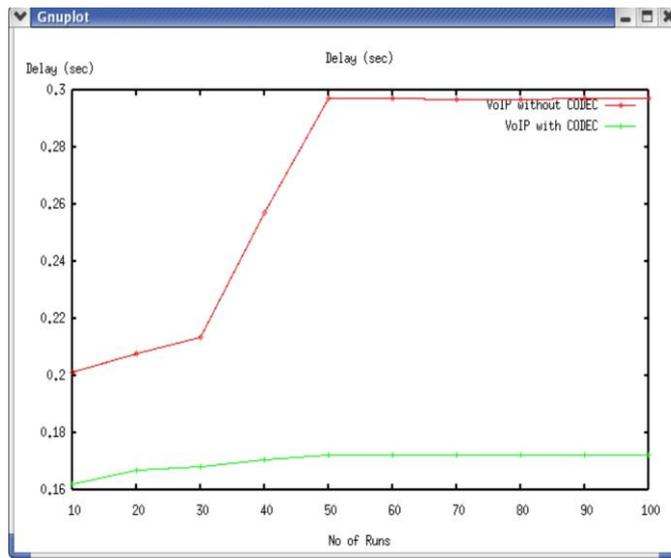
Fig.11 Packet delay for VoIP without codec and VoIP with codec when simulation is run 100 times
