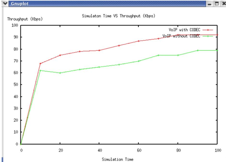
Fig. 6 Throughput for VoIP in MANET without codec and with codec
