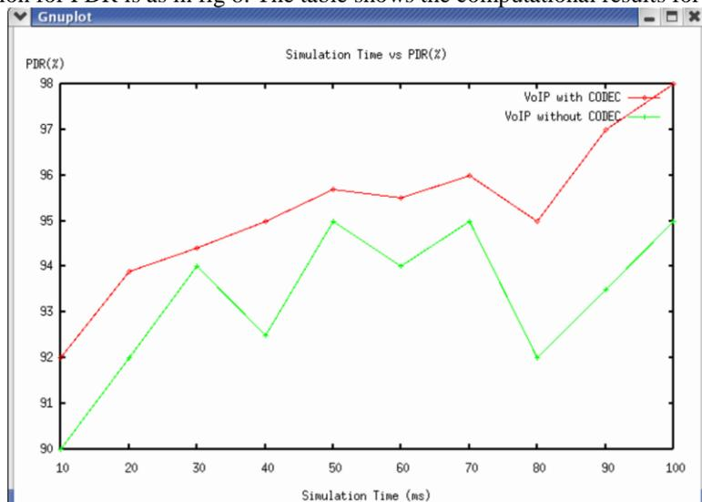
Fig. 8 PDR for VoIP without codec and VoIP with codec
