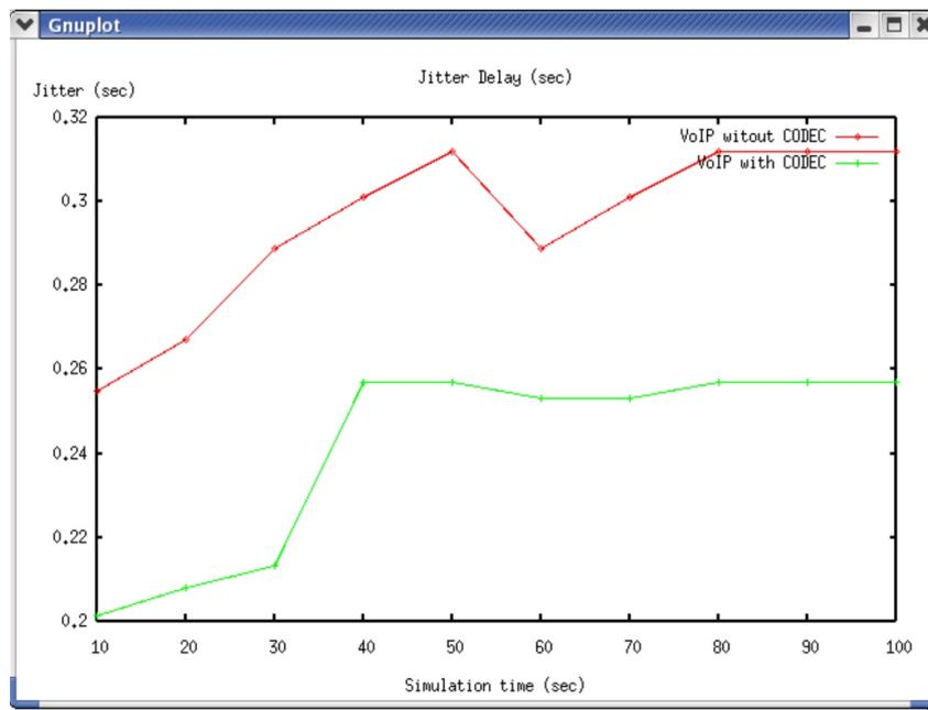
Fig. 7 Jitter for VoIP without codec and VoIP with codec
