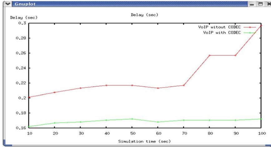
Fig. 10 Packet delay for VoIP without codec and VoIP with codec
