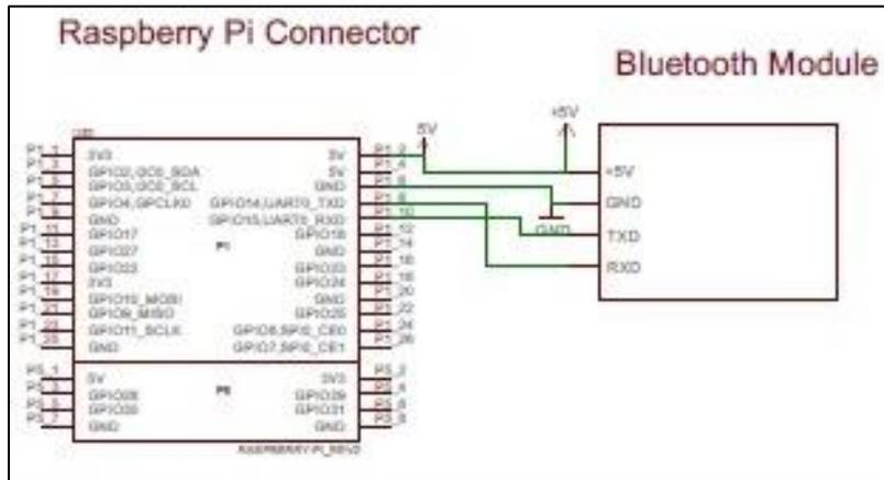
Figure. 3 Raspberry pi connected with Bluetooth module
