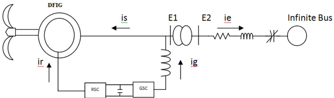
Figure 1. Wind turbine model
