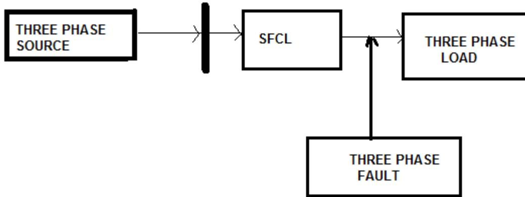
Fig 3.0 Superconducting Fault Current Limiter connected in series transmission line
