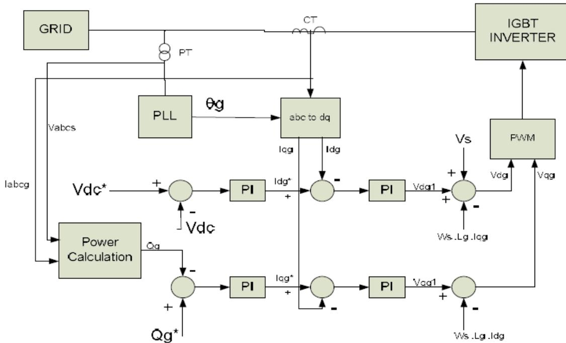
Figure 2. The Grid-Side Converter (GSC)
